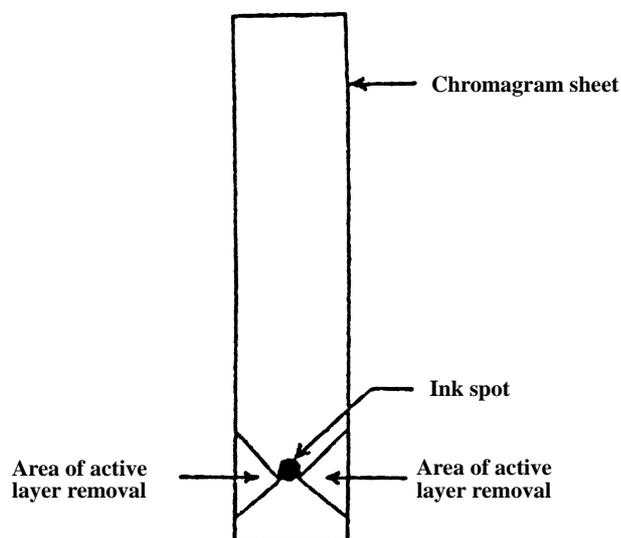
Fig. 1 Pattern for active layer removal
