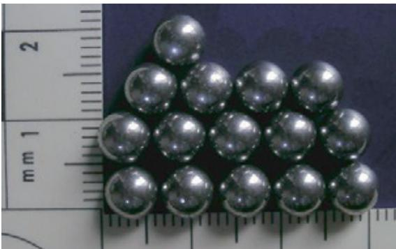
**Fig. 6** The 6 mm caliber steel pellets used for test firings.
