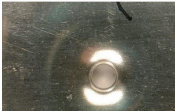
**Fig. 7** A complete penetration bullet hole on the witness plate from the test of case 1 air rifle.
