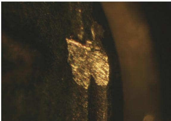
**Fig.3** An inconclusive comparison image of ejector marks on an imitation (right) and a genuine (left) cartridge case.
