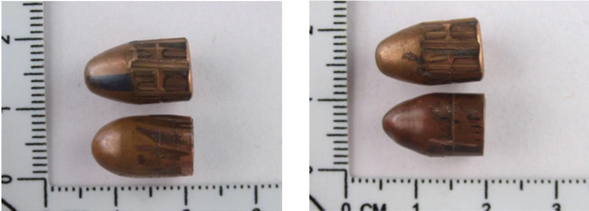
**Fig.11** The rifling patterns on fired GR (top left and right), IW (bottom left) and IA (bottom right) bullets.
