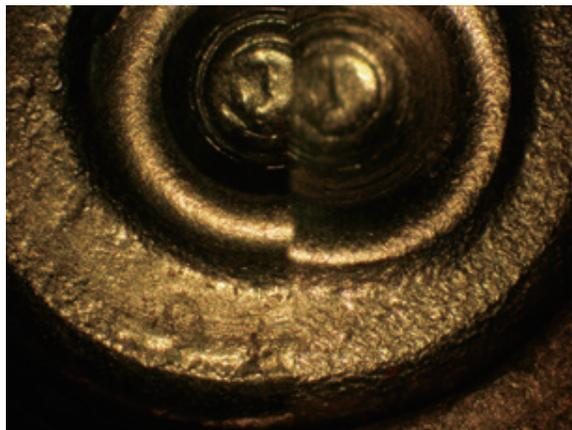
**Fig.5** An inconclusive comparison image of breech-block marks on an imitation (right) and a genuine (left) cartridge case.
