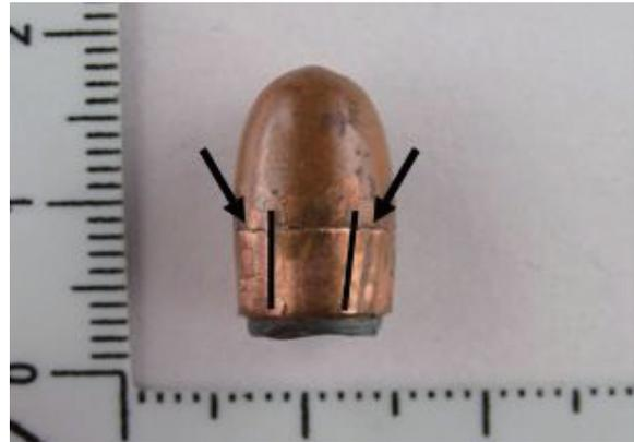
**Fig.13** Different rifling impressions with varied tilt angles formed on the same fired IW bullet as indicated by the arrows and lines.
