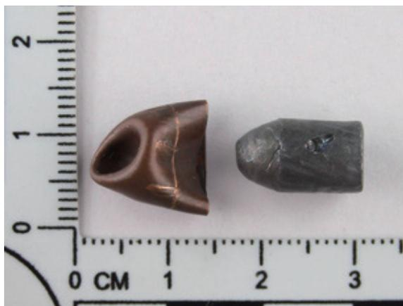
**Fig.10** A separated metal jacket (left) and lead core (right) of a fired imitation bullet.
