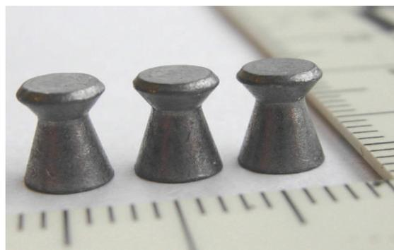
**Fig. 4** Diabolo type pellets with a caliber of 4.5 mm
