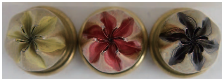
Fig. 4 The crimps and varied color codes on case mouths of blank cartridges.
