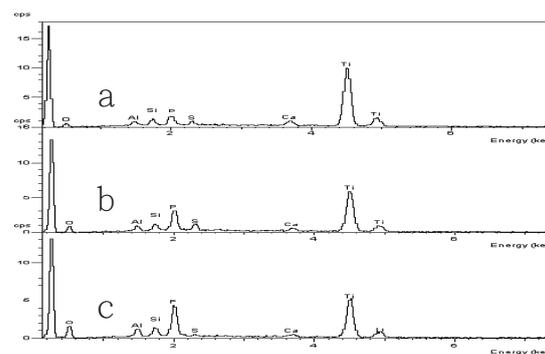
**Fig. 7** The pre-combustion EDS spectra of mixed fire retardant (type B-2)-architectural (type G-1) coatings at volume mixing ratios of 1:2 (a), 1:1 (b), and 2:1 (c).
