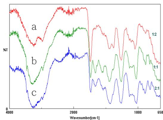
**Fig. 6** The pre-combustion IR absorption spectra of mixed fire retardant (type B-2)-architectural (type G-1) coating at volume mixing ratios of 1:2 (a), 1:1 (b), and 2:1(c).
