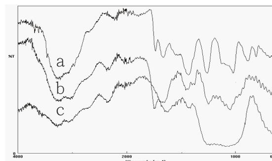
**Fig. 4** The IR spectra of fire-retardant coating, type B-2, before combustion (a), boundary layer after combustion (b), and char layer after combustion (c).
