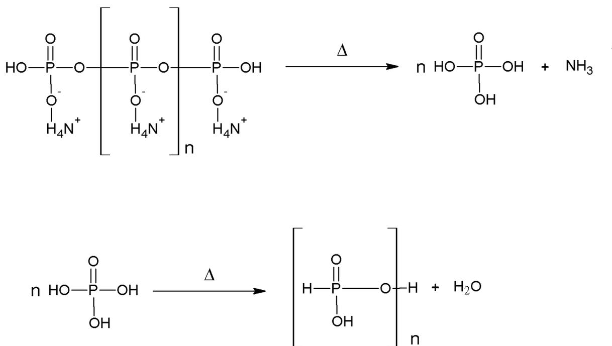
**Scheme 1** Thermal decomposition of ammonium polyphosphate [2].
