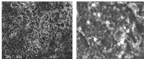
**Fig. 1** The surface appearance of Type A-1 (left) and B-1 (right) in the SEM ( $\times 750$ ).
