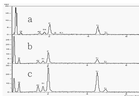
**Fig. 5** The EDS spectra of fire-retardant coating, type B-2, before combustion (a), boundary layer after combustion (b), and char layer after combustion (c).
