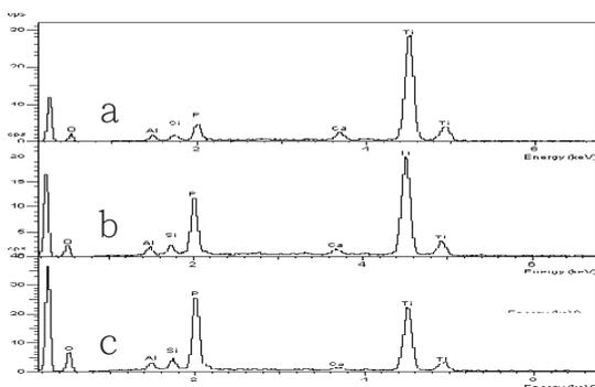
**Fig. 9** The post-combustion EDS spectra of mixed fire retardant (type B-2)-architectural (type G-1) coating at the volume mixing ratio of 1:2 (a), 1:1 (b), and 2:1 (c).
