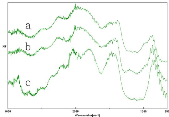
**Fig. 8** The post-combustion IR absorption spectra of mixed fire retardant (type B-2)-architectural (type G-1) coatings at volume mixing ratios of 1:2 (a), 1:1 (b), and 2:1 (c).
