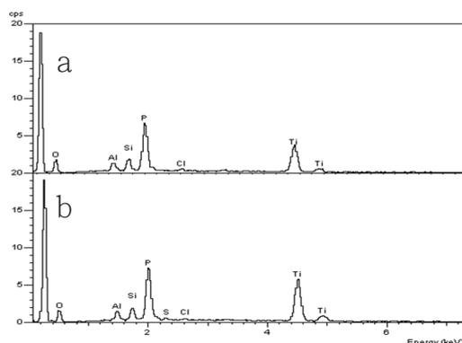
**Fig. 3** The EDS spectra of types B-1 (a) and B-2 (b).
