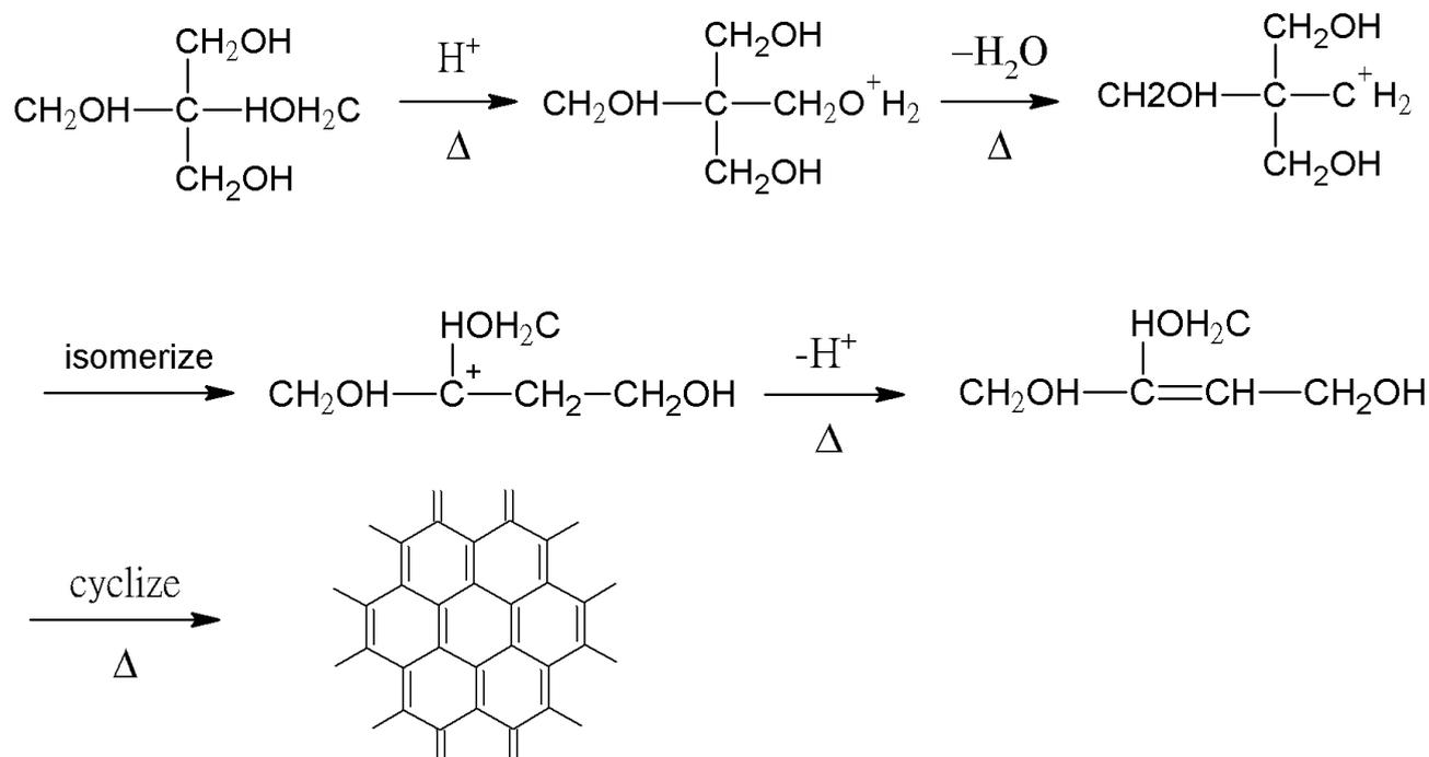
**Scheme 3** Reaction of char formation under combustion [2].
