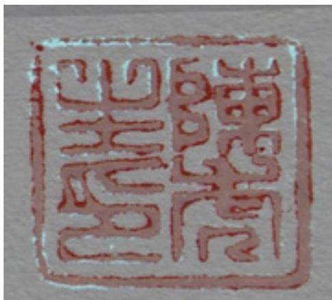
**Fig. 3** Overlay checking to the impression of the original seal and the impression obtained from the original seal with excessive ink on the seal face and with heavy pressing pressure.
