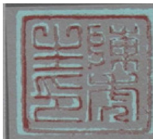
**Fig. 5** Overlay checking to the impressions of the original seal and the reproduced seal made by photoelectric automatic engraver.
