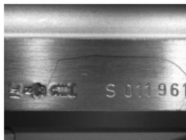
**Fig.5** The "JH" proof marks on the slide of Sig Sauer pistol indicate the year of 1987
