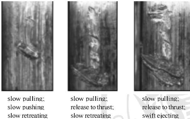
**Fig. 9** J-shape extractor marks are different in length on unfired conditions. (For Beretta 92 FS or the series)
