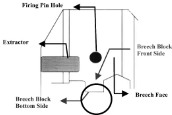
**Fig. 4** The breech block bottom side move over the upper surface of the top round cartridge.
