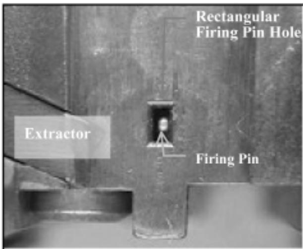
**Fig.16** The rectangular firing pin hole of Glock pistol.
