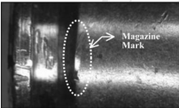
**Fig.2** The magazine scratch mark of H & K USP Compact, being vertical to axis of cartridge case.
