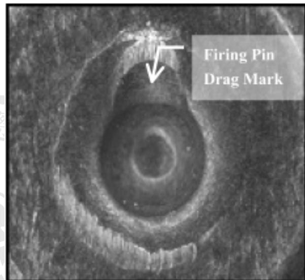
**Fig.15** Firing pin drag mark on the upper north side (12 o'clock position) of firing pin impression.
