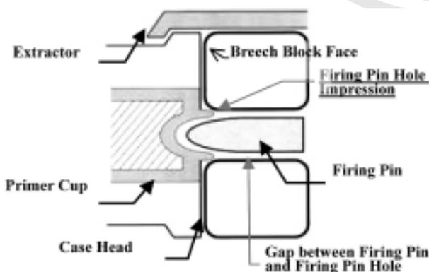
**Fig.18** Mechanism of forming firing pin hole impression.
