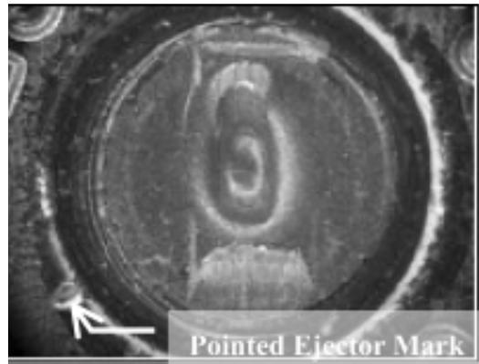
**Fig.10** The pointed ejector mark near the primer of cartridge at 8-9 o'clock position. (Glock 17 )
