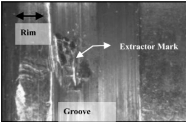
**Fig. 8** Irregular extractor mark in the groove of the unfired cartridge case. ( Sig-Sauer P226 )
