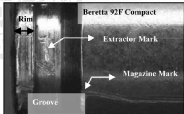
**Fig. 7** J-shaped extractor mark in the groove of the unfired cartridge case. ( Beretta model 92FS)
