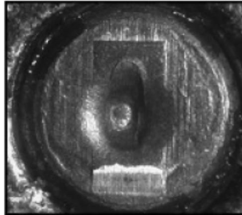
**Fig.20** Vertically straight line breech face impression produced by the Glock Model 17
