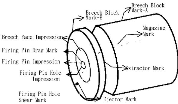
**Fig.1** Various tool-marks left on spent cartridge cases (from 9mm auto-loading pistols)
