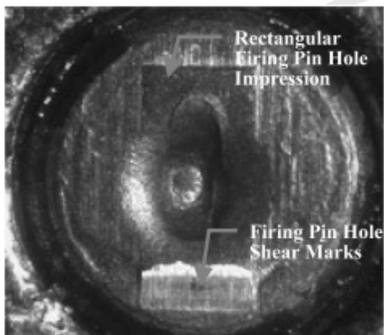
**Fig.17** Rectangular firing pin hole impression on the spent cartridge cases produced by Glock pistols.
