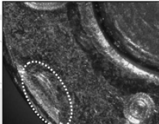
**Fig.11** The fan-shaped ejector mark at 8 o'clock near the cartridge rim. (Beretta 92FS)
