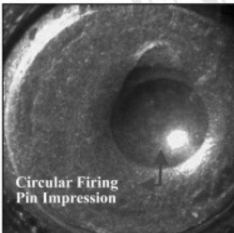
**Fig.14** Circular firing pin impression impinged on primer of spent cartridge cases. (Beretta pistols)
