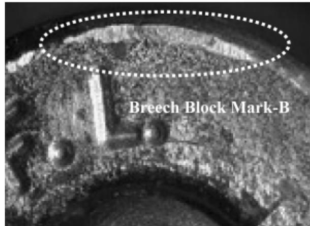
**Fig. 6** Impact pattern of breech block mark – B on upper edge of cartridge case.
