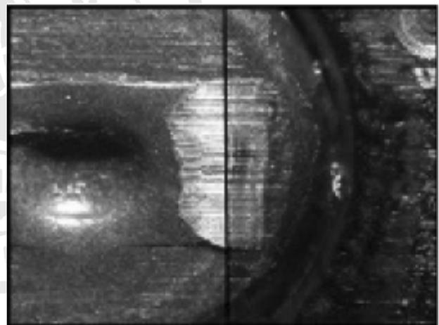
**Fig.19** A match comparison of firing pin hole shear mark of two fired cartridge cases with identical Glock 17 pistol.
