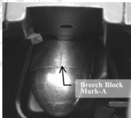
**Fig. 3** Breech block mark-A ---when the bolt moves backward once a shot has been discharged, the breech block bottom side slides over the upper surface of the top cartridge in the magazine. (Parallel skid mark)
