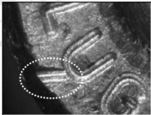
**Fig.12** The triangular shaped ejector mark are near the rim of cartridge at 8 o'clock position. (Sig-Sauer P228)
