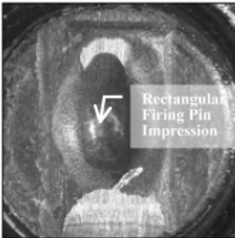
**Fig.13** Rectangular firing pin impression impinged on primer of spent cartridge cases. (For Glock 17 & 19)
