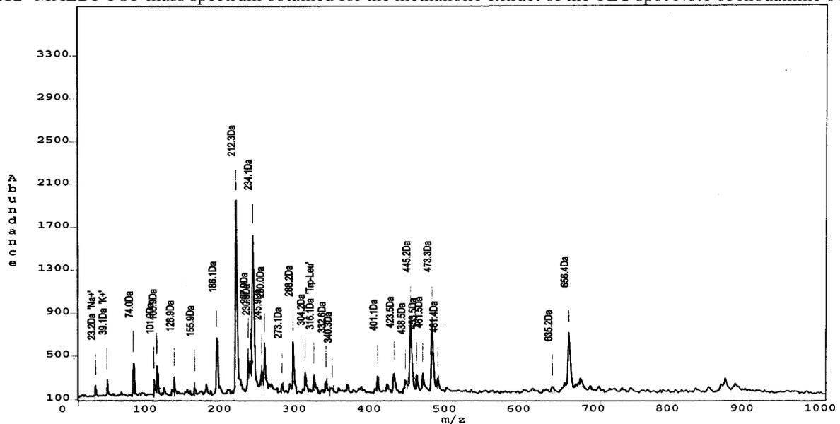
Fig.13 MALDI-TOF mass spectrum obtained for a methanolic extract of TLC spot No.2 of rhodamine 6G dye
