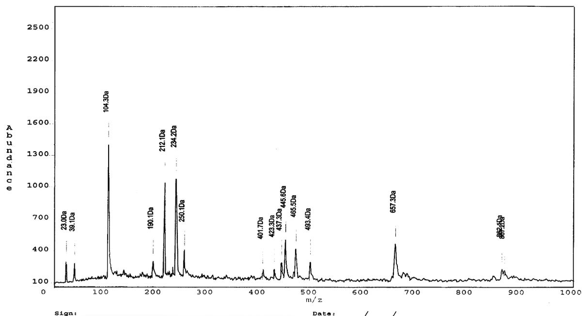
**Fig.1** MALDI-TOF mass spectrum of the matrix, CHC.
