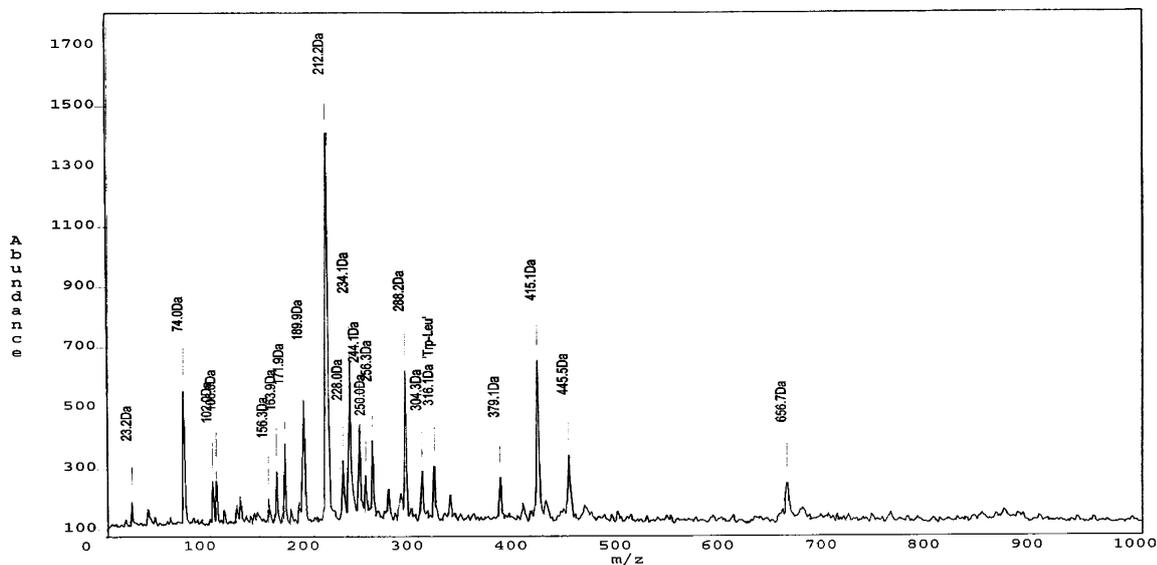
Fig.10 MALDI-TOF mass spectrum obtained for the methanolic extract of the TLC spot No.4 of Staedtler 430 M ink.
