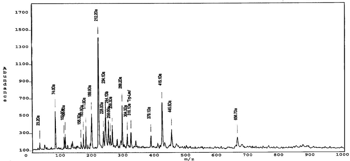
Fig.12 MALDI-TOF mass spectrum obtained for the methanolic extract of the TLC spot No.1 of rhodamine 6G dye
