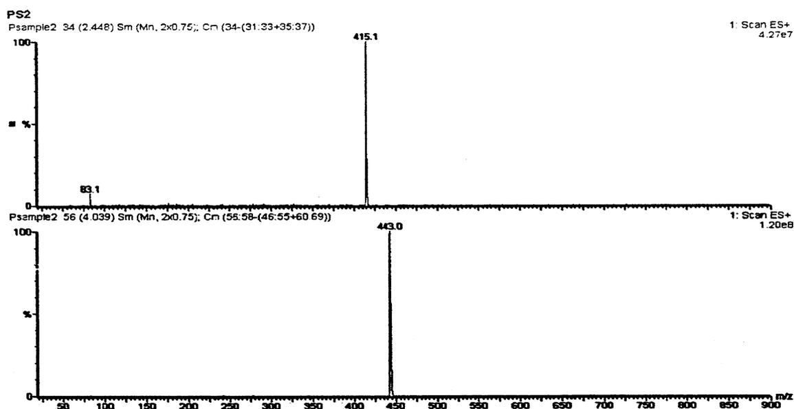
Fig.16 ESI mass spectra obtained for the methanolic extracts of the TLC spots No.1 and No. 2 of Bic red ink.
