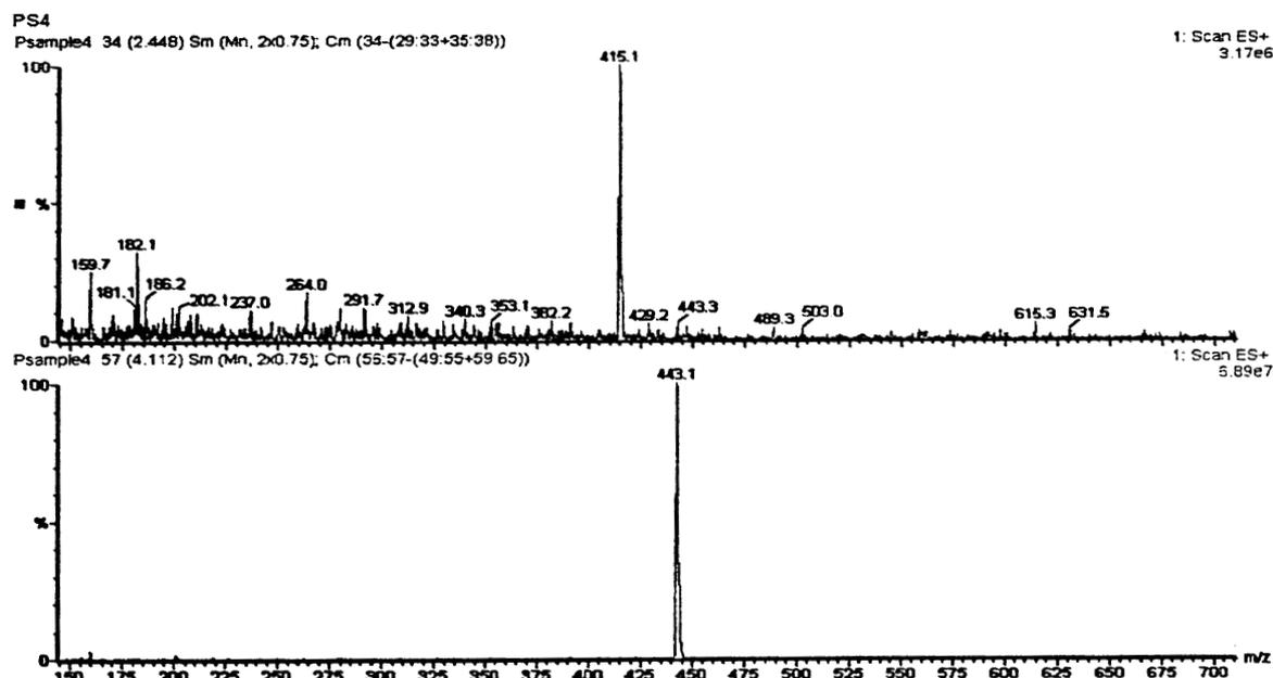
Fig.17 ESI mass spectra obtained for the methanolic extracts of the TLC spots No.1 and No.2 of rhodamine B dye
