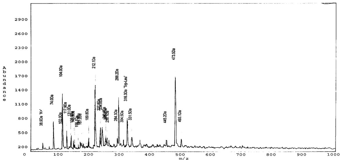
Fig.8 MALDI-TOF mass spectrum obtained for the methanolic extract of the TLC spot No.2 of Staedtler 430 M ink.
