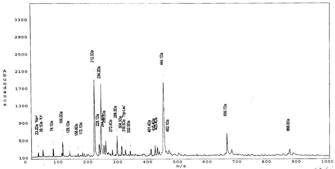
Fig.14 MALDI-TOF mass spectrum obtained for the methanolic extract of the TLC spot No.3 of rhodamine 6G dye
