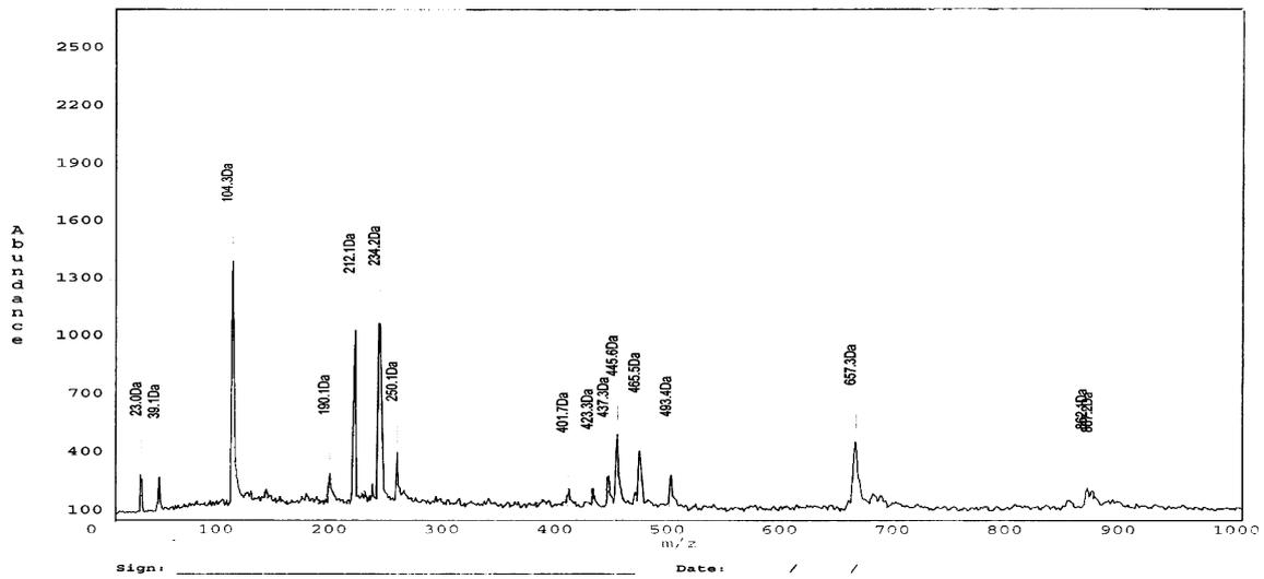
**Fig.2** MALDI-TOF mass spectrum obtained for the methanolic extract of blank carbonless paper
