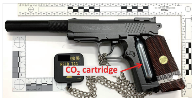
Fig. 2 Photograph of the actual-case liquefied CO 2 airgun.
