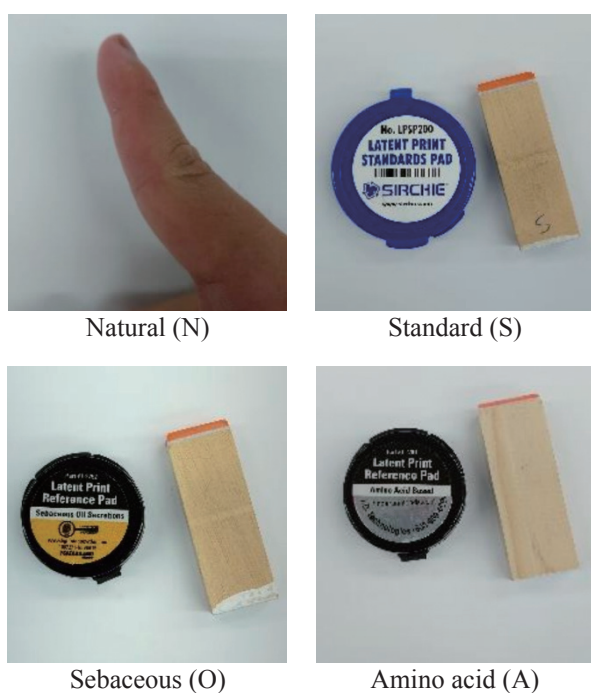
Fig. 1 Representative images of the four fingermark compositions deposited on substrates. (N) Natural fingermark from a live donor; (S) Standard, (O) Sebaceous, and (A) Amino acid fingermarks deposited using rubber stamps derived from scanned inked prints.
